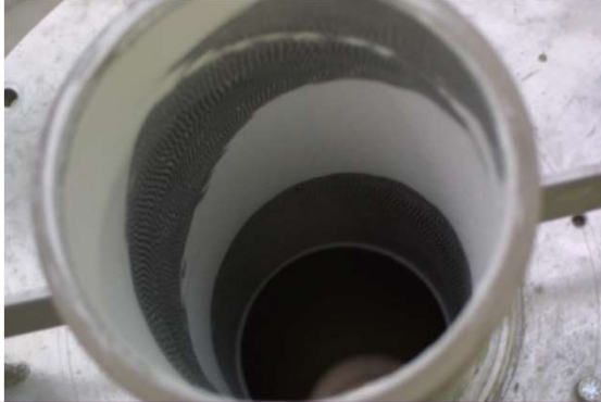
View in the cone of a cyclone with deposits on the wall
