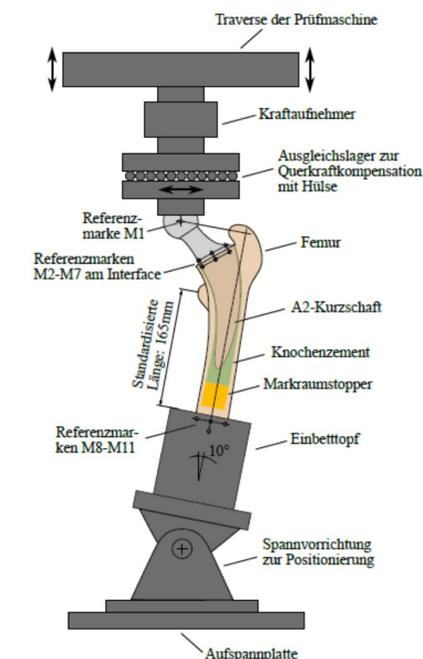
Figure 2: Fatigue tests of hip endoprostheses
