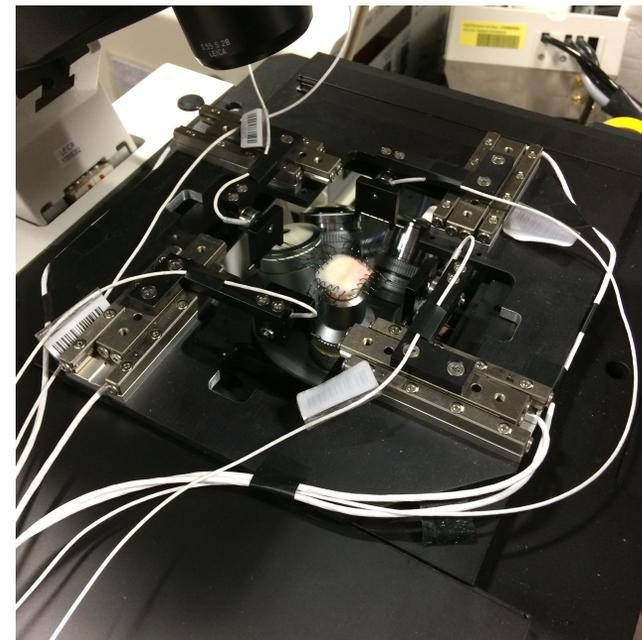
Device for biaxial extension tests
