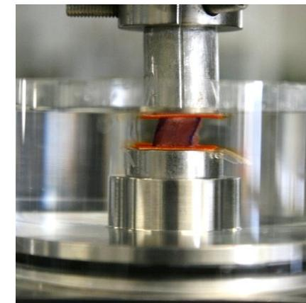
Figure for topic 1: Representative image of the experimental set-up used to test myocardium under shear
